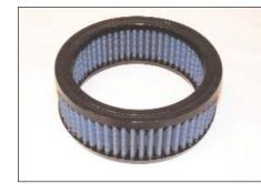
Filter Number Product Style Inner Wire Height (in) Outside Length/Diameter (in) Outside Width (in) Inside Diameter (in) Opening Style General Applications EaAM23 Circular Style Air Filter Yes 2.188 6.000 N/A 4.625 N/A S & S Teardrop Housing
